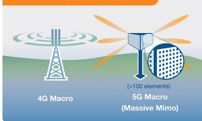
4G sector base station and 5G base station with a new multi element massive MIMO antenna array. The overall physical size of the 5G base station antenna is expected to be similar to a 4G base station antenna.
